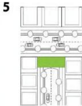
5 T-Junctions were avoided for returnable plots by providing urban plug-ins.
